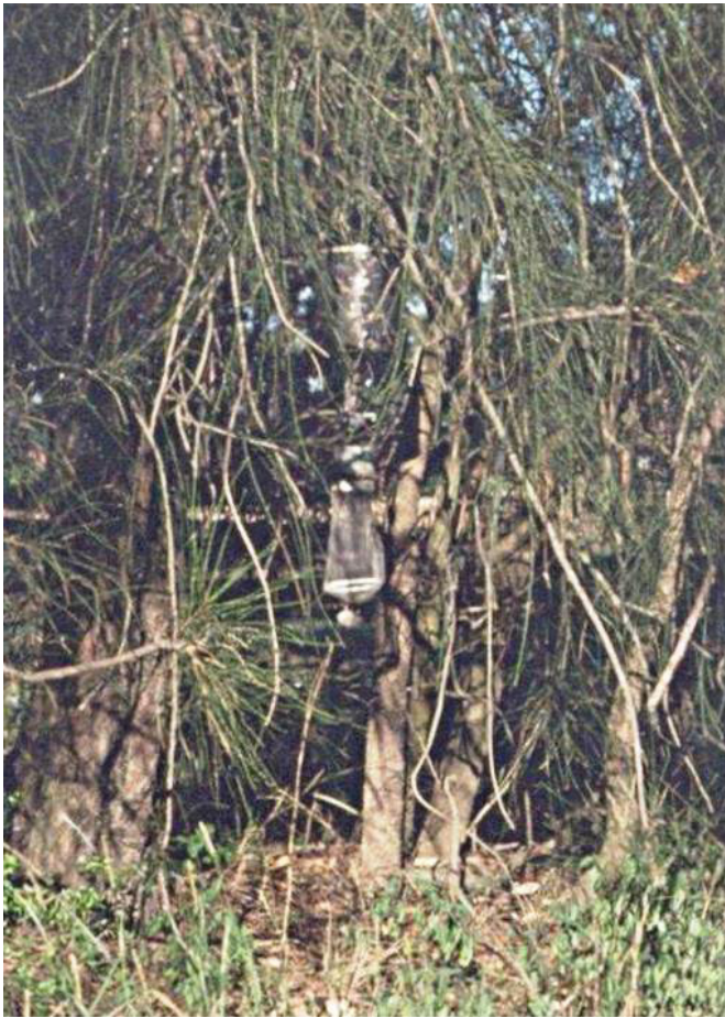
Figure 2.11.6. A wetland will provide mosquito habitat. Mosquitoes may carry diseases, which can be passed on to humans. Monitoring a wetland includes sampling for pest species. Entomologists use traps consisting of dry ice (CO 2 ), an LED and a small fan to entice mosquitoes into a fine mesh mosquito net beneath the trap.
