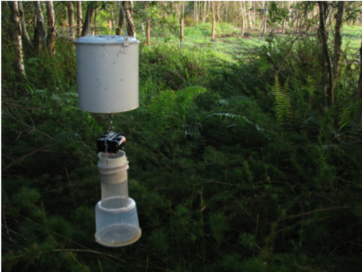
Figure 3.6.8. The foundation for effective mosquito management is a good surveillance program. The most commonly used mosquito traps in Australia use carbon dioxide to attract mosquitoes. The abundance and diversity of mosquitoes collected provides an assessment of mosquito risks and the effectiveness of mosquito control programs. Specimens can also be tested to determine if they are infected with any mosquito-borne pathogens. (Photo: Cameron Webb, Medical Entomology, Pathology West – ICPMR Westmead.)
